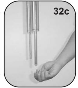
33. With rebound damper shaft in the fully-extended position, measure and pour or inject 130cc/ml (+/- 5cc/ml) 5wt suspension oil into upper tube (through crown) (fig 33).
