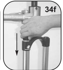
Press the damper down until the upper damper o-ring contacts the upper tube threads. Turn the damper clockwise and thread into upper tube (fig 34f).. This will protect the upper damper o-ring as it passes the upper tube threads. Do not push straight down; this will damage the compression damper o-ring seal. Hand-thread top cap into upper tube (fig 34f) and tighten to 60 in-lb with a 24mm socket wrench (fig 27a).
