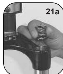
22. Spray entire spring assembly with isopropyl alcohol. Wipe all grease and oil from top cap, spring and shaft. Apply grease to outside of entire coil spring and spring isolator.
