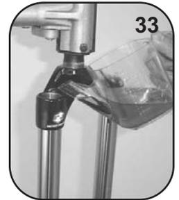
34. Coat the new compression damper u-cup seal with suspension oil.
