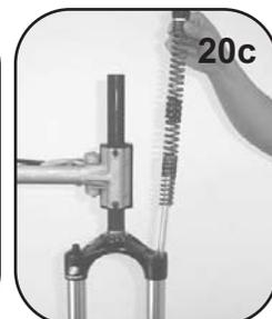
21. Remove U-Turn negative spring assembly from upper tube (fig 21). You may need to remove fork from bicycle workstand and turn upside down to remove. Clean and re-install.
